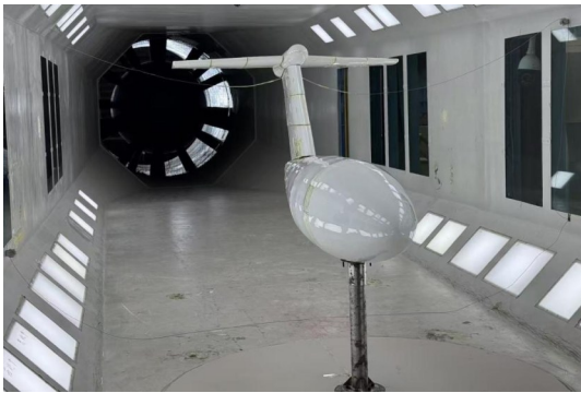
图9 T尾颤振模型在风洞中的安装状态 Fig. 9 The mounting configuration of the T-tail flutter model in the wind tunnel
